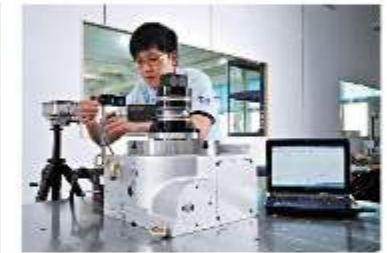
Laser measuring equipment (Indexing precision testing)
