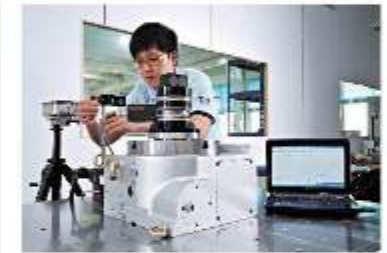
Laser measuring equipment [Indexing precision testing]
